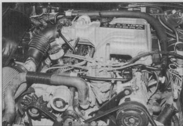
1 We began the installation on Mike Broder's '90 LX, which features a stock short-block, ported Canfield aluminum heads, and a Cobra upper/lower.
