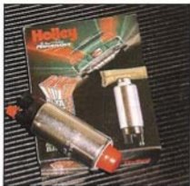
The 190 lph pump (#12-901) flowed 176 lph, but would not run above 65 psi without popping off externally.
