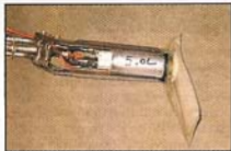
The pump that started it all, the 88-lph 5-liter pump, checked in at 91 lph on our test bench at 13 volts and 40 psi.
