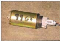
The stock 2V 4.6 pump flowed much better than the 5.0 pump, registering 158 lph at 40 psi and 13V.
