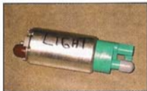
The supercharged 5.4 Lightning pump flowed just 149 lph, surprising given the power rating of the force-fed Modular V-8.
