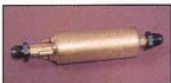
After running the in-the-tank pumps, we turned our attention to the inline fuel pumps. This T-rex pump from Vortech flowed 162 lph at 40 psi.
