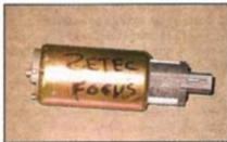
We even took the liberty of flowing the stock Zetec Focus pump, which responded with 143 lph at 40 psi.
