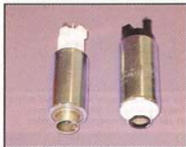
Though similar in shape, the early positive displacement (5.0 and early 4.6) electric fuel pumps and the later turbine (late 4.6) pumps differ in design. The two are not interchangeable, though turbine pumps can be used in positive displacement applications.
