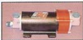
The highest flowing pump of the test belonged to Barry Grant. The King Sumo pump flowed 608 lph at 40 psi and 13 volts and an amazing 759 lph at 40 psi and 17 volts. Figure on a dedicated wiring harness for the King Sumo, as the amp draw was pretty significant on the bad boy.
