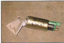
The SVT Focus pumped really cranked out the flow, registering 217 lph. The SVT Focus topped the list of production fuel pumps.
