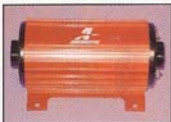
The Aeromotive 11104 inline fuel pump was quite impressive at 512 lph at 40 psi and 13 volts.
