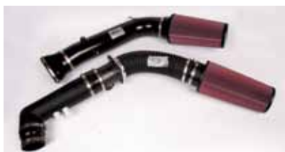
▲ Jim Bell was running flow tests on various 4.6 Two-Valve modular intakes when we visited. At bottom is a stock 4.6 Mustang GT unit. As the duct taped number indicates, it flows a modest 536 cfm on KB's flowbench. The elephant trunk at top is the KB intake ducting from their standard 2.1-liter Two-Valve kit. It flows substantially better at 782 cfm, but that's still not enough to support major power initiatives.
