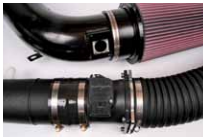
▲ Airflow can be unintuitive at times. The corrugated tubing on the standard air inlet is much more restrictive than it looks as the corrugations trip and tumble the air, not to mention its small mass air meter housing.
