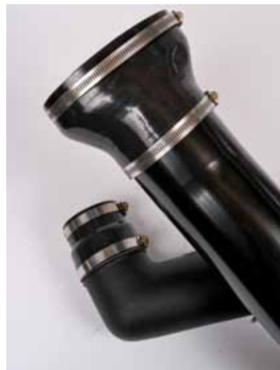
▲ Another not so subtle clue to the Mammoth inlet tube's power capacity is its belled throttle body adapter hose. The standard kit, by comparison, necks down to mate with its throttle body.
