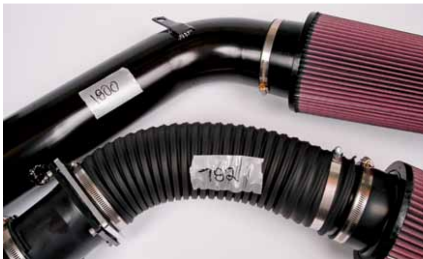
▲ Airflow can be unintuitive at times. The corrugated tubing on the standard air inlet is much more restrictive than it looks as the corrugations trip and tumble the air, not to mention its small mass air meter housing.
