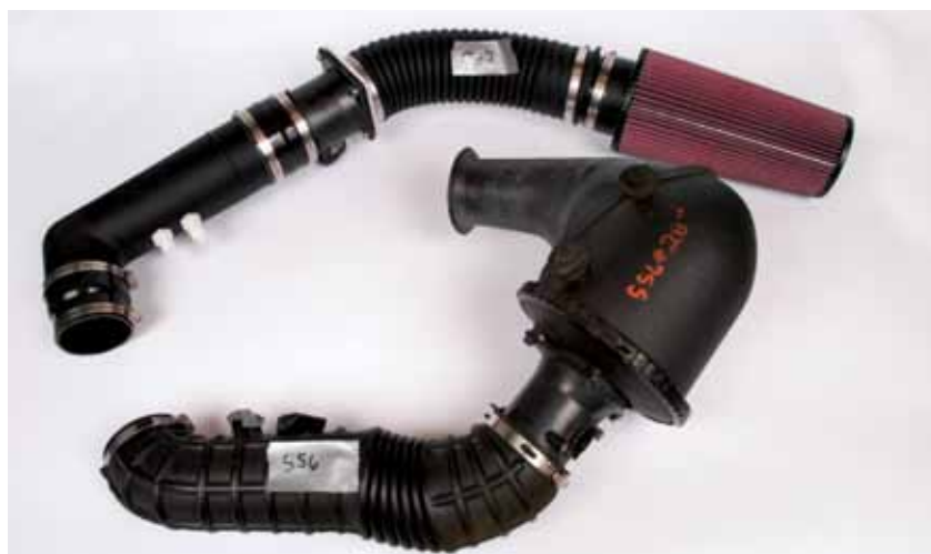
▲ Jim Bell was running flow tests on various 4.6 Two-Valve modular intakes when we visited. At bottom is a stock 4.6 Mustang GT unit. As the duct taped number indicates, it flows a modest 536 cfm on KB's flowbench. The elephant trunk at top is the KB intake ducting from their standard 2.1-liter Two-Valve kit. It flows substantially better at 782 cfm, but that's still not enough to support major power initiatives.
